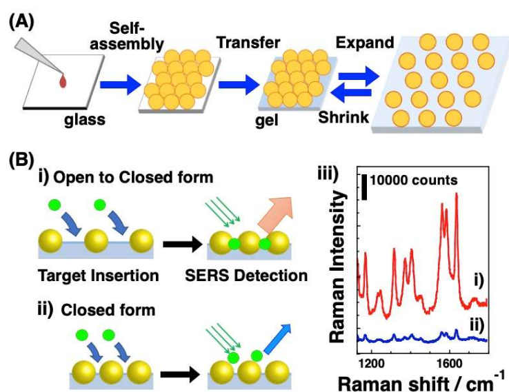
Figure 1. (A) Schematic illustration of the preparation of gap tunable AuNP arrays on the hydrogel and (B) SERS detection using active gap tunable AuNP arrays; i) scheme of active gap approach, in which gap is open for the target insertion and then closed for SERS detection, ii) scheme of conventional approach, in which gap is closed for target insertion and SERS detection, and iii) SERS spectra of cytochrome c measured by these approaches.
