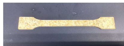
fig.1 Sample prepared for strength testing
