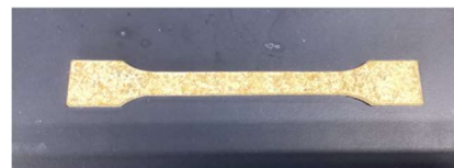
fig.1 Sample prepared for strength testing.
